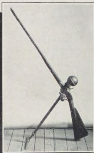
Air gun made by Priestley which fires twelve shots without recompression.
