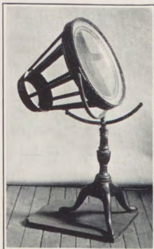
Large compound burning glass with 16 and 7 inch lenses, used by Priestley in discovery of oxygen.
