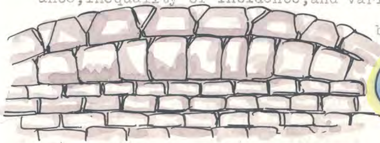
CROSS-SECTION OF PORTION OF TELFORD SUB-PAVEMENT LAID ON ROLLED EARTH FOUNDATION, SHOWING METHOD OF WEDGING STONES AND PACKING CHIPS INTO VOIDS AND INTERSTICES.
