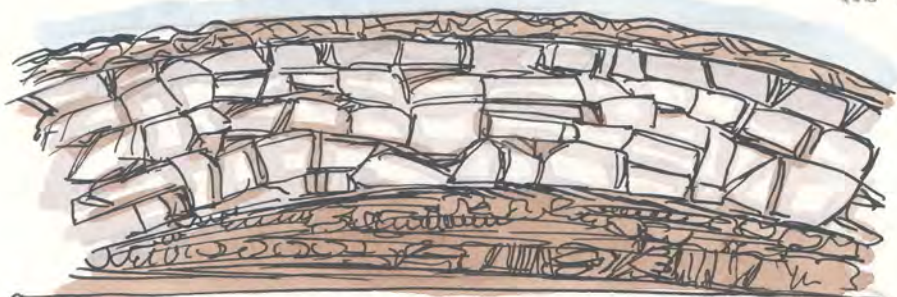
CROSS-SECTION OF MACADAM AND TELFORD ROADWAY LAID ON AN EARTH AND ROCK FOUNDATION, AND MADE SOLID AND PERMANENT BY HEAVY ROLLING.
