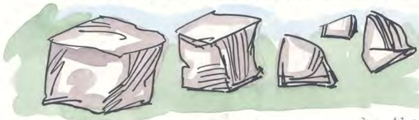
CUBE-SHAPED STONES OF PROPER SIZE FOR TOP LAYER OF MACADAMIZED ROADWAY.
